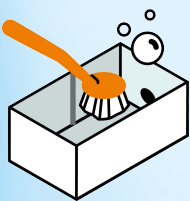
3. Clean fluff box
